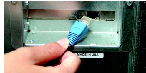
Figure 3-3: Connect the Ethernet Network Cable
